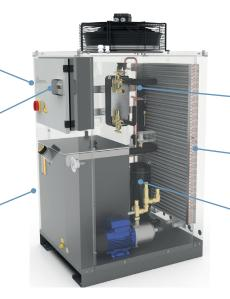
ATMOSPHERIC HYDRAULIC CIRCUIT made of non-ferrous material, equipped with automatic bypass valve. The HDPE storage tank is thermally insulated and equipped with level indicator and front loading and drainage connections. Centrifugal pumps P3/P4/P6/P5 inverter (optional)
